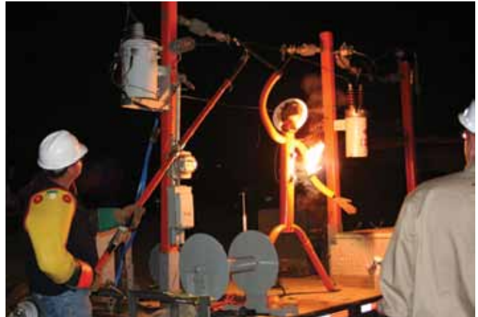
Sanden Simons shows the affect of high voltage power traveling thru the body.
